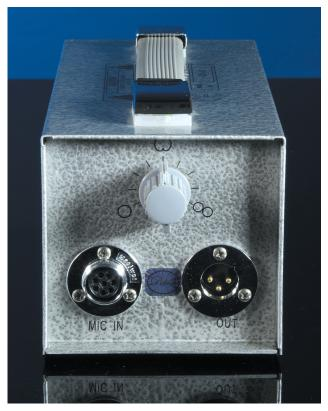
Unlike the original power supply, which offered continuously variable pattern selection, the Peluso has nine discrete settings, which range from omnidirectional, through cardioid, to figure-of-eight.
